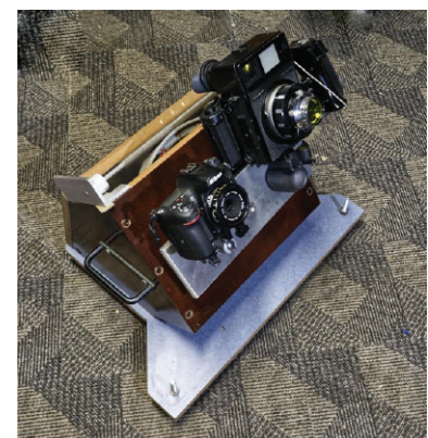
Figure 4 The Complete assembly with two cameras mounted The unit as constructed, was larger than that needed to support a camera (or two as shown in Figure 4) and will be applied to a fork mounted Newtonian telescope (a future project).
