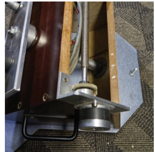
Figure 2 Stepper motor and drive train
